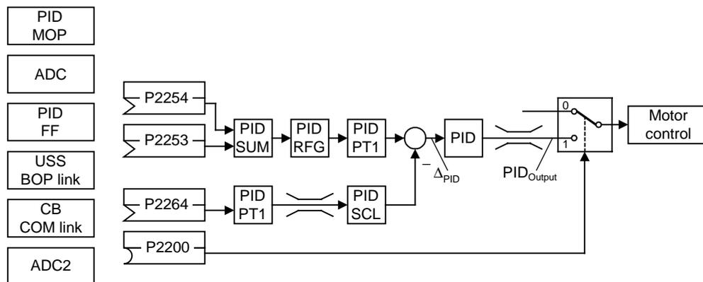
This parameter allows the user to select the source of the PID setpoint. Normally, a digital setpoint is selected either using a fixed PID setpoint or an active setpoint.
