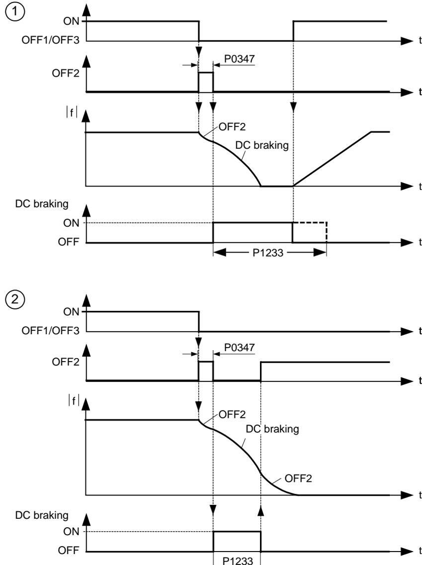
Parameter P1232 still controls the level of DC injection.
