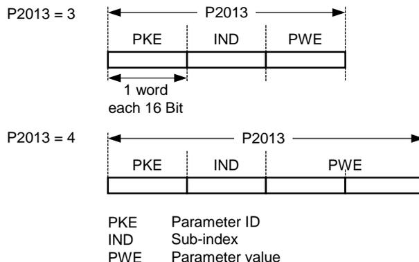
P2013 = 3, fixes PKW length, but does not allow access to many parameter values. A parameter fault is generated when an out-of-range value is used, the value will not be accepted but the inverter state will not be affected. Useful for applications where parameters are not changed, but MM3s are also used. Broadcast mode is not possible with this setting.
