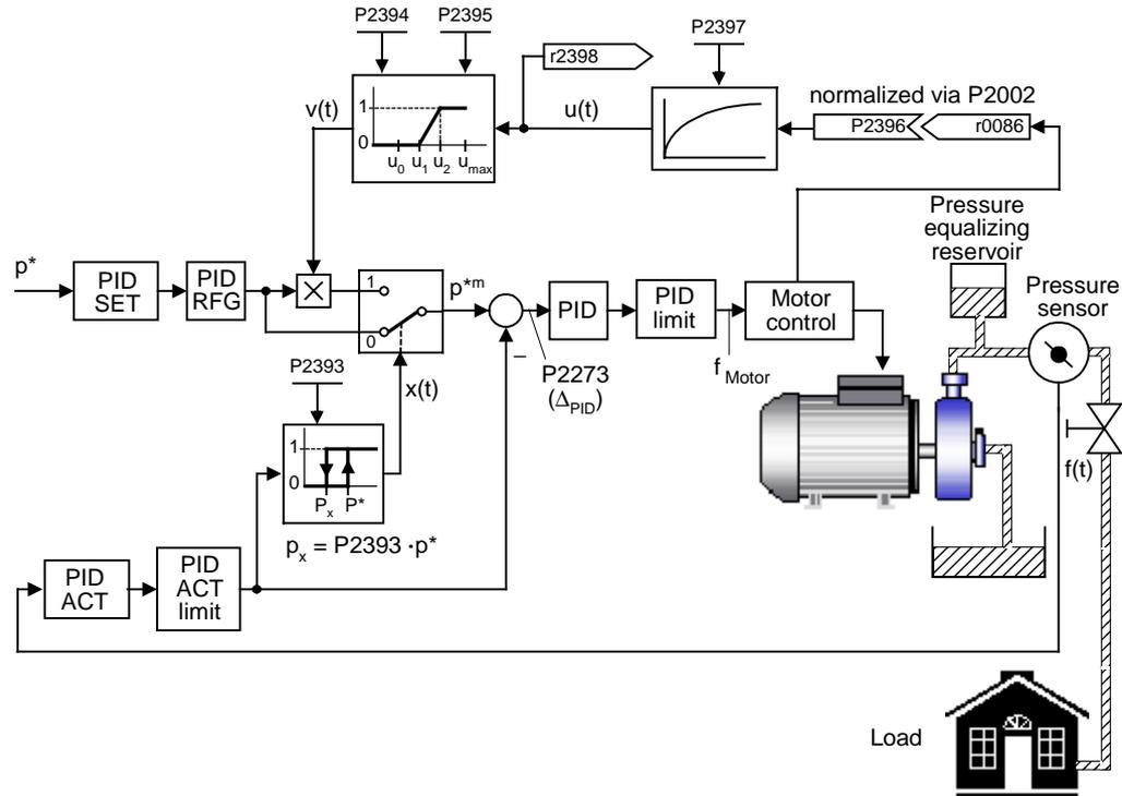
If the active current falls below the normalized threshold P2395, then the setpoint is linearly decreased as a function of the active current.
