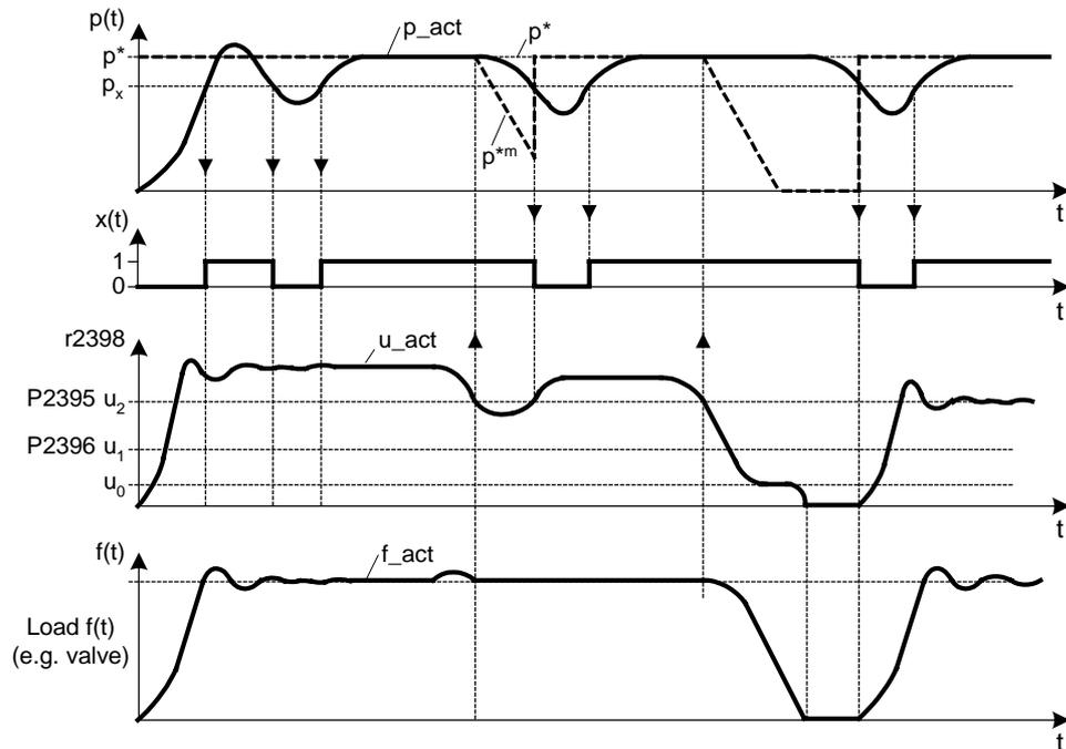
If the actual value falls below threshold  $p_x$  after the motor was shutdown, the inverter automatically powers-up again without having to toggle the ON command.
