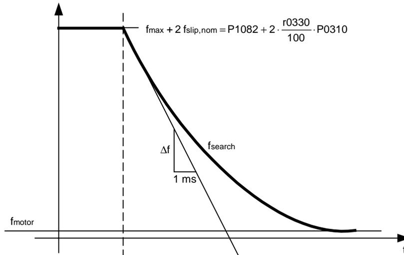
$$P1203 [\%] = \frac{\Delta t [\text{ms}]}{\Delta f [\text{Hz}]} \cdot \frac{f_{\text{slip,nom}} [\text{Hz}]}{1 [\text{ms}]} \cdot 2 [\%]$$
